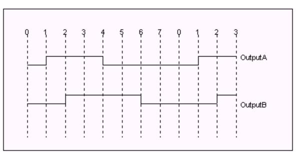
This can be replaced by an 8-step sequencer. Step 1 (e.g "Seq1:1") turns ON and latch Output A using [Latch] function, Step 2 turns ON and latch Output B, Step 4
