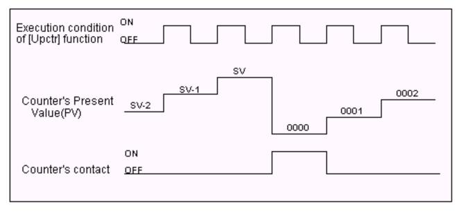
Each time when the execution condition of an [Upctr] function changes from OFF to ON, the present value of the designated counter is affected as follow:
