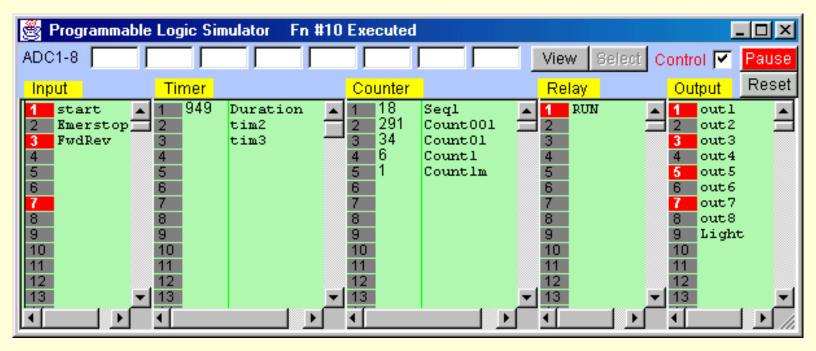
An I/O or internal relay bit that has been turned ON is indicated by a RED color rectangular lamp that simulate a LED being turned ON. You can pause the logic simulator at any time by pressing the <Ctrl-P> key or clicking on the [Pause] button. Likewise the simulator engine can be reset by clicking on the [Reset] button.
