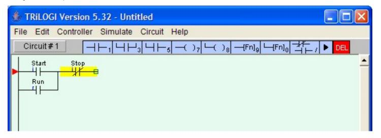
7. We will now connect a relay coil "Run" to the right of the "Stop" contact. Click on the coil. Select "RUN" label from the "Relay" table. Remember that an input can never be used as a coil. Fortunately, TRILOGI is smart enough not to call up the "Inputs" table when you are connecting a coil, to avoid unintentional errors.
