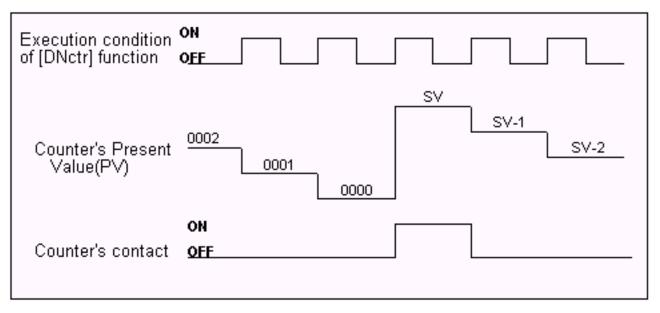
Each time when the execution condition of a [DNctr] function changes from OFF to ON, the present value of the designated counter is changed as follow:
