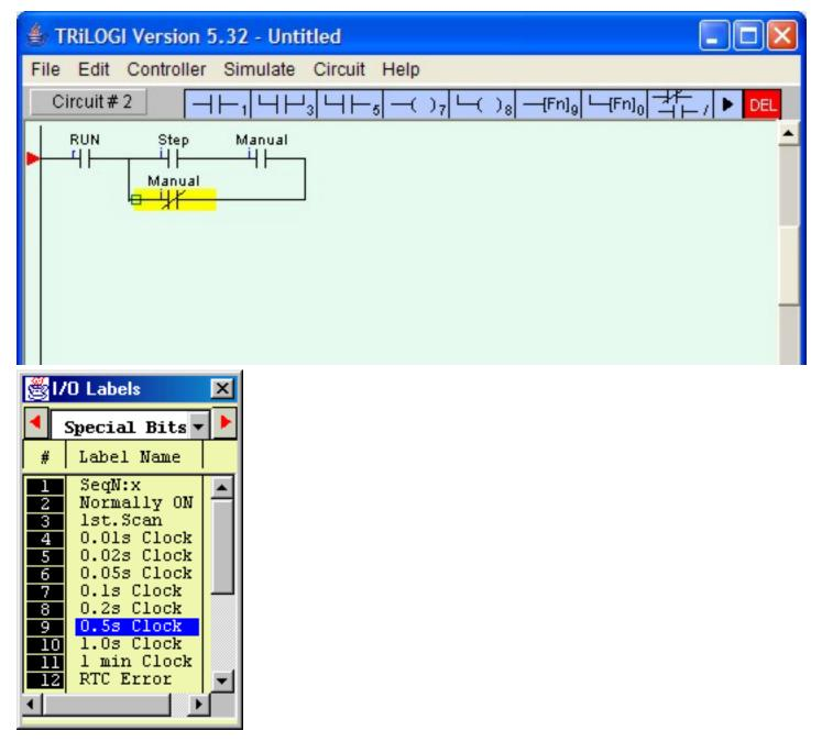
5. Next, we want to insert the special bit "Clk:0.5s" to the left of the "Manual" contact. Press the <SHIFT> key to move the insertion point to the left end of the highlight bar as shown above. Then left-click on the left icon to create a normally-open contact. Scroll the I/O table to the "Special Bits" table and select the item: "0.5s Clock". The parallel branch would have been completed by now.
