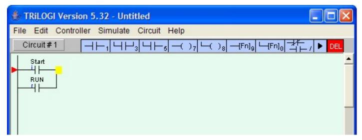
Note: In TRiLOGI Version 5.32 or higher, the highlight bar will move to the junction if you click on the dark green insertion point on the "Start" contact.
