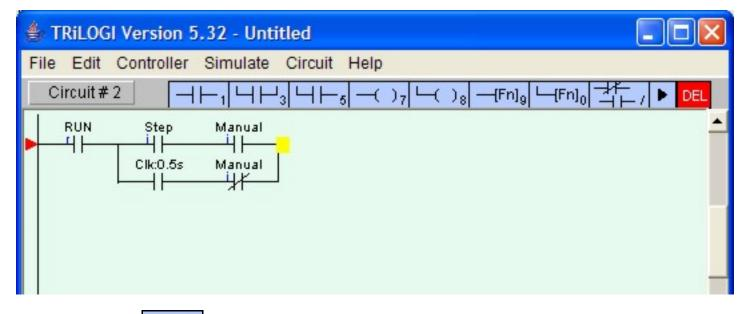
7. Now, click on the <code>\_\_\_\_[Fn]</code> icon to insert a special function coil. A popup menu will appear for you to select the desired special function. Click on the item "4.[AVseq]-Advance Sequencer" to insert the Advance Sequencer function [AVseq].
