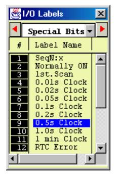
The "Special Bits" table is located after the "Counters" table and before the "Inputs" table. Then click on the "SeqN:x" item to insert a sequencer bit. You will be prompted to select a sequencer from a pop-up menu. Choose the desired sequencer (1 to 8) and another dialog box will open up for you to enter the specific step number for this sequencer.
