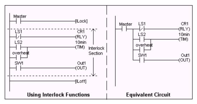
Note that [ILoff] is the only function that does not need to be energized by other program elements. When you use one or more [ILock] functions, there must be at least one [ILoff] function before the end of the program. Otherwise the compiler will warn you for the missing [ILoff]. The logic simulator always clears the Interlock at the end of the scan if you omit the [ILoff] function.
