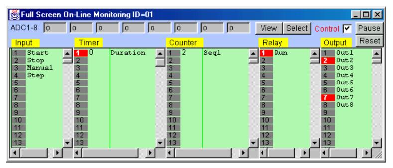
The Full Screen Monitoring screen comprises 5 columns: Input, Timer, Counter/Sequencer, Relay, and Output. With the exception of the Relay table which contains up to 512 elements, all other columns contain 256 elements each and each one has a vertical scroll bar. You can use the mouse to scroll each column independently to locate the desired I/O.
