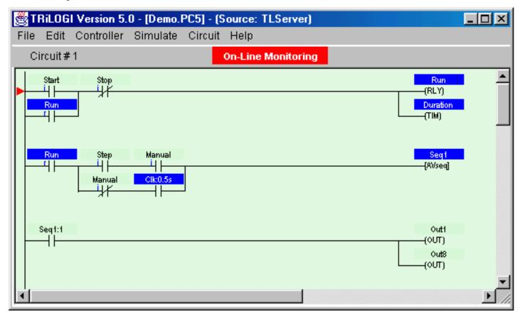
• Note that whether the highlight is turned is based strictly on the logic state of an element. You will have to interpret whether the contact is opened or closed by examining if it is a normally-open (N.O.) or a normally-closed (N.C.) contact. A highlighted N.C. contact means that the contact is opened, whereas a highlighted N.O. contact means that the contact is closed.
