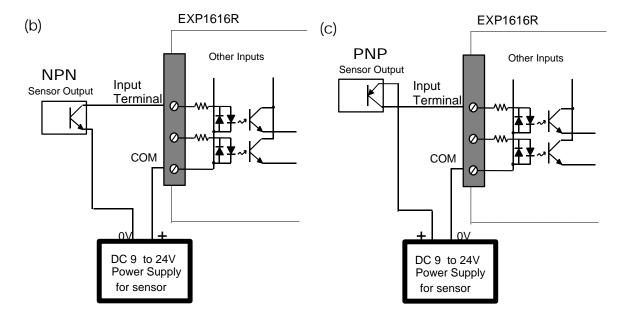
Figure 3 - EXP1616R Input Wirings
