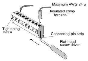
Figure 2 - Removing screw terminal block
