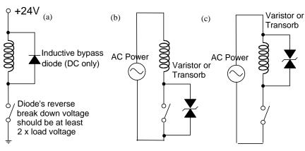
Figure 5 - (a) Inductive snubber circuit - DC load only. (b), (c) Inductive snubber circuit - AC/DC load.
