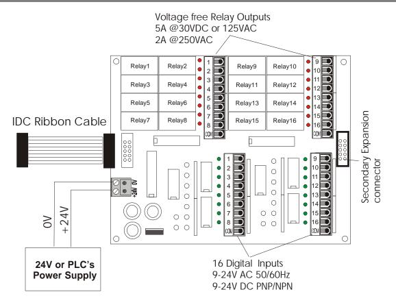
Figure 1 - 32 I/O Expansion board for T100MD PLC
