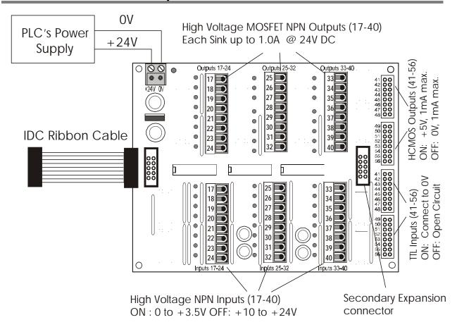
Figure 1 - 40 I/O Expansion board for T100MD PLC
