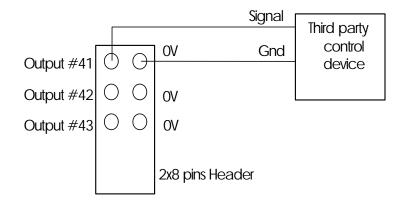
Figure 4 - Interfacing HCMOS Outputs to External Logic Device.
