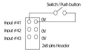
Figure 3 - Close the switch will turn ON a TTL Logic-Level Input.
