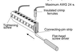
Figure 2 - Removing Screw Terminal block
