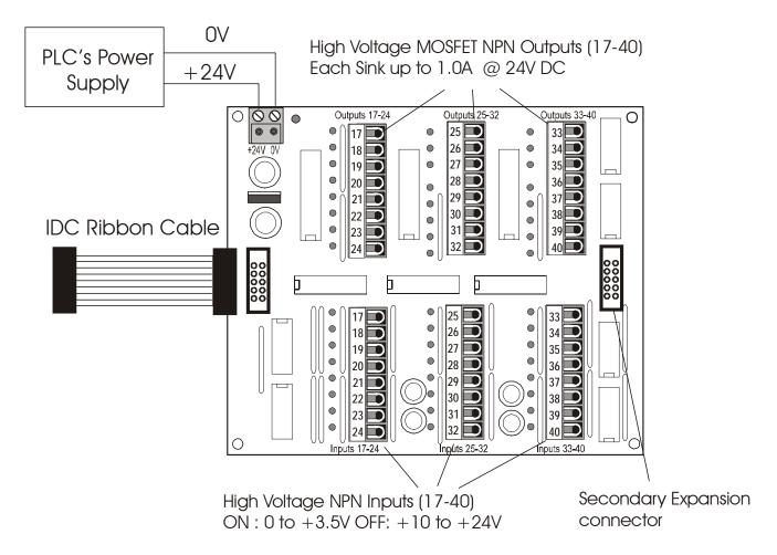
Figure 1 - 24 Inputs, 24 Outputs I/O Expansion board for FMD & F-series PLC
