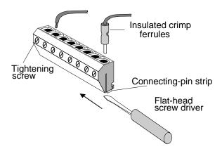
Figure 2 - Removing Screw Terminal block
